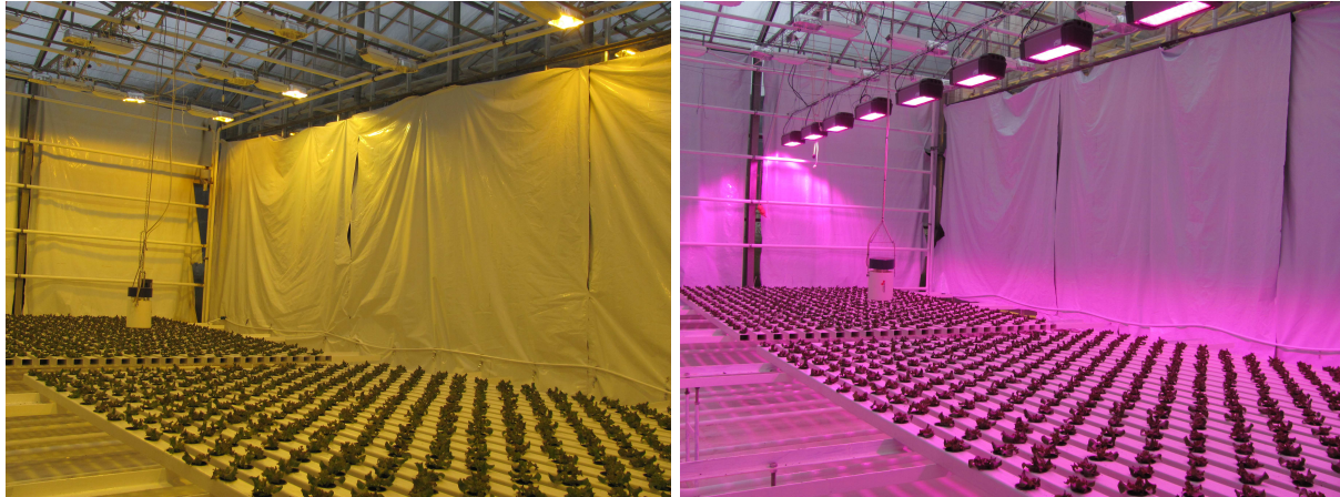
Fig. 7a: Salad one week after growing in the NFT channels (left: HPS, right: LED, experiment A).
